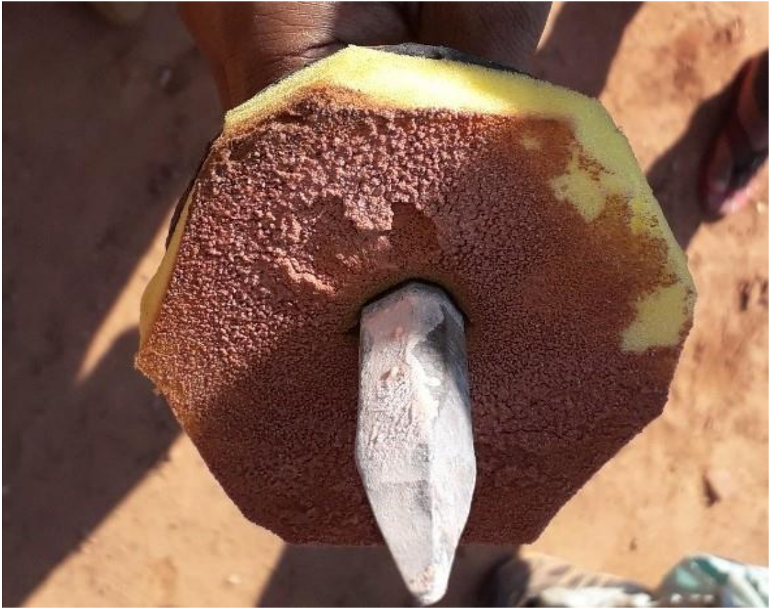
Fig 10 Close view of dust captured by Karauli Tanki
