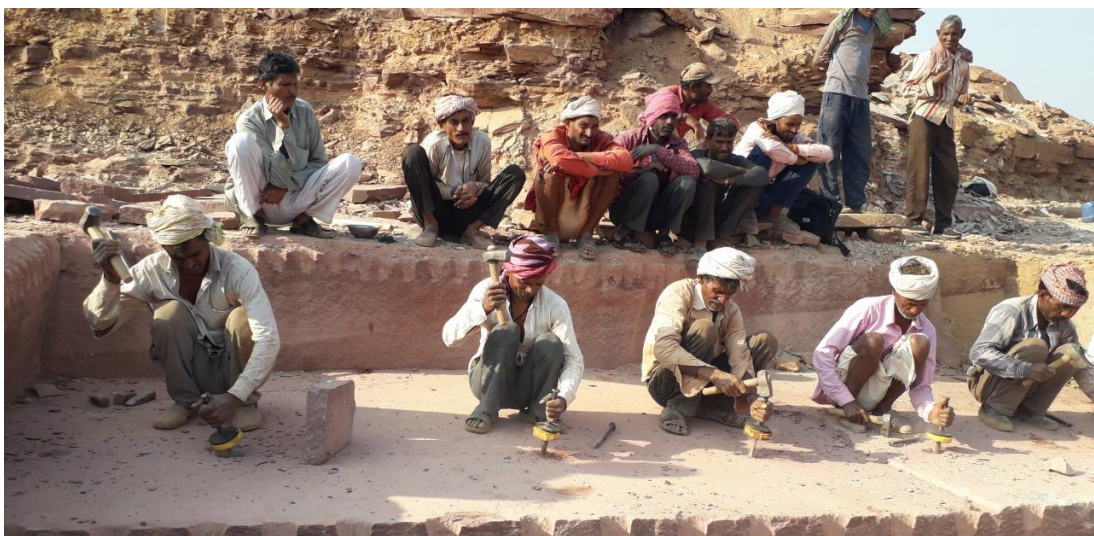
Fig 8 Demonstration of use of Karauli Tanki by Mine Workers
