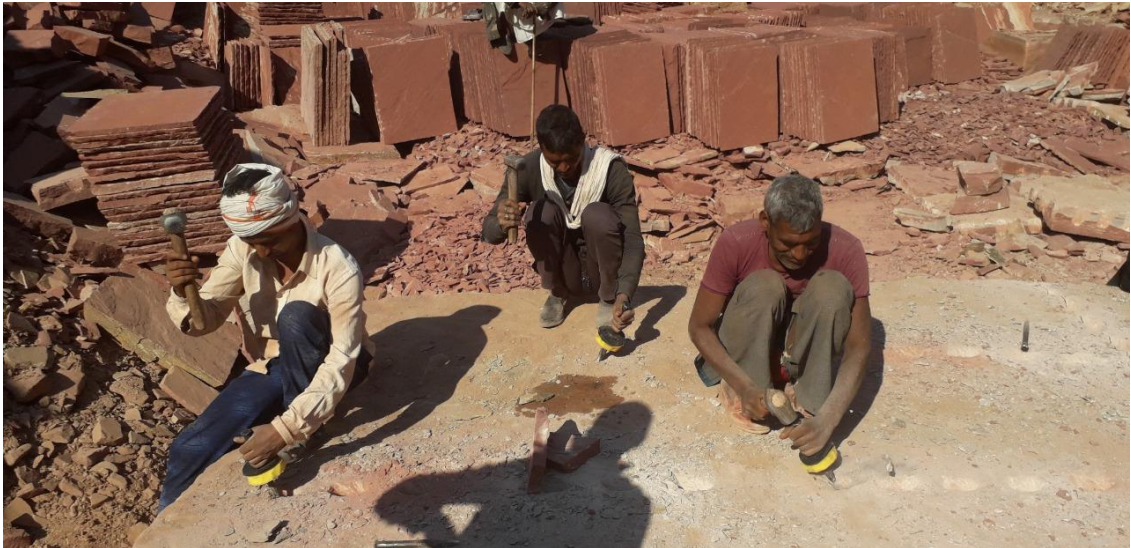
Fig 8 Mine Workers using “Karauli Tanki”
